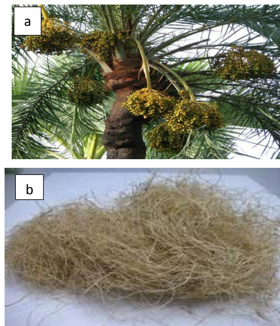
Fig.1: (a) Schematic picture of the date palm ( Phoenix dactylifera L. ) tree and (b) date palm trunk fibers (DPTFs)
