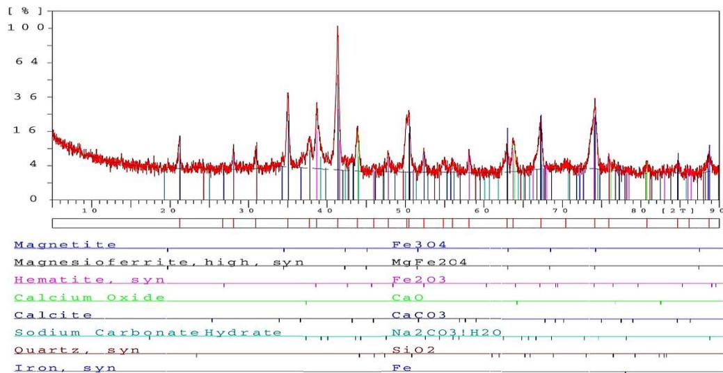
Fig. 2: XRD patterns of collecting dust in the cyclone
