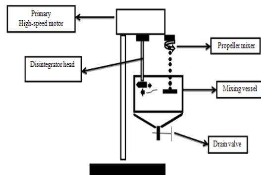
**Fig 1:** High-speed and high shear double –mixer set
