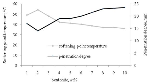
**Fig 1:** The effect of bentonite wt% variations on both SP and penetration degree (2 wt% SBS)
