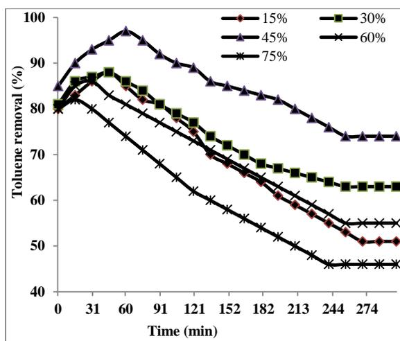
Fig. 6: Effect of relative humidity on toluene removal efficiency (toluene concentration of 300 ppm and UV intensity of 17 w/m<sup>2</sup>)
