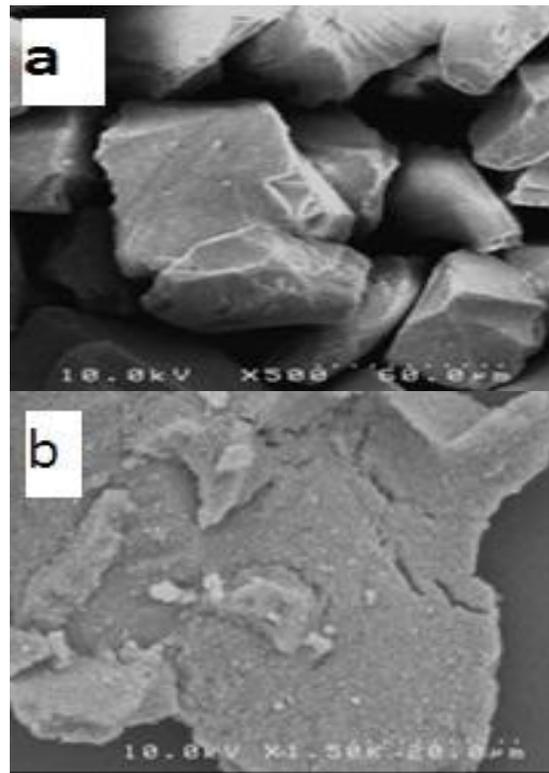
**Fig. 2:** Micrograph prepared by a scanning electron microscope from the silica gel bed (a) and catalyst  $\text{TiO}_2/\text{SiO}_2$  (b)
