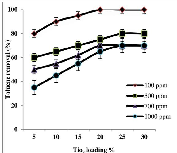
**Fig. 3:** Toluene photocatalytic oxidation efficiency using TiO<sub>2</sub> / SiO<sub>2</sub> catalyst (catalyst; 5 to 30 wt.%, toluene concentration; 100 to 1000 ppm, apparent gas velocity; 2 l/m, humidity; 45%).
