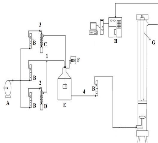
**Fig. 1:** Schematic diagram of the fluid bed reactor along with a system for providing the pollutant-specific concentration and relative humidity. Air Blower (A), Rotameter (B), Water Impinger (C), Toluene Impinger (D), Mixing Enclosure (E), Moisture Sensor (F), Fluid Bed Reactor (G), Gas Chromatography (H)
