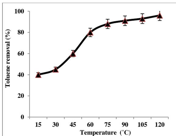
Fig. 5: Effect of reactor column temperature on toluene removal efficiency (300 ppm toluene concentration - relative humidity 45% - intensity of UV radiation 17 w / m<sup>2</sup>)
