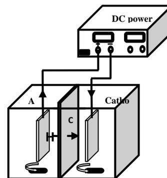
Fig. 1: Schematic diagram of the bioelectrochemical reactor
