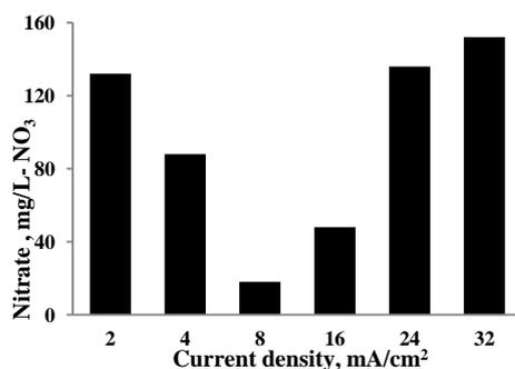
**Fig. 2:** Effect of current density on bioelectrochemical nitrate reduction ( $\text{NO}_3^- = 200 \text{ mg L}^{-1} \text{NO}_3^-$ , Time=8h)
